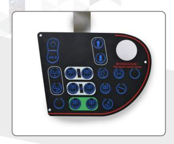
to provide the management of electro-, pneumo- and hydro- vehicles systems. Controllers allow to represent the status of the executable functions, alarm and other messages on the built-in displays and on the backup multicolored light panels (including invisible signal mnemonic symbols), and provides sound\voice backup of warning and alarm messages.
