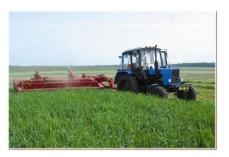
Mower-conditioner KPP-4,2 "PALESSE CT42" is intended for mowing of grass with simultaneous squashing of mowed crops and putting them into swath to the stubble. Also it can be used for grass mowing without squashing with gathering of mowed mass into swath. Operates with 1,4 drawbar category tractors.
