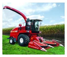
KVK-800 "PALESSE FS80-2" is intended to mow down maize of any ripeness stage and other high-stemmed crops, to pick up slightly dried seeded and natural grass from swaths with simultaneous chopping and loading of the mass into transport trailer.
