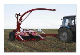
Pull-type harvester KDP-3000 "PALESSE FT40" is intended for harvesting maize, including wax-ripened and complete ripeness maize, sorgo, sunflower and other tall-stalked crops, mowing green crops, picking-up mass from swaths of prewilted sowed and natural grass with simultaneous crushing and loading into the transporter-wagon.
