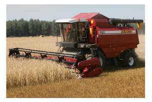
The combine harvester is intended for direct and windrow harvesting and it can also be used for harvesting of of maize, sunflowers, leguminous, cereal crops, grass and rape seeds using special equipment.
