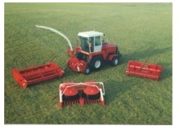
harvesting Forage complex "K-G-6 PALESSE" is intended for harvesting of maize, including wax and full-ripened maize, other high-stemmed crops, also for mowing green and picking-up slightly dried, sowed and natural grass from swaths, chopping and transporter-wagons. loading into Forage harvesting complex "K-G-6 PALESSE" includes universal power vehicle, chopping
