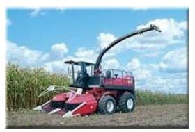
KSK-600 "PALESSE FS60" is intended for mowing down maize of any ripeness stage, sunflower and other highstemmed crops, mowing down grass and picking up slightly dried seeded and natural grass from swaths with simultaneous chopping and loading of the mass into transport trailer.
