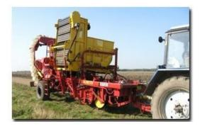
Semi-coupled potato harvesting combine PKK-2-05 "PALESSE PT25" with a bunker and a sorter desk is intended for harvesting of potato on light and mediumtextured soils in moderate climate zones of potato growing, except mountainous, with the field grade limit up to 4°.
